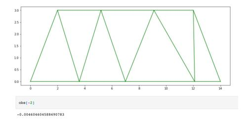
Which one can compare with an initial design that has bigger middle node displacement of -0.005108382058368501, hence worser stiffness.
